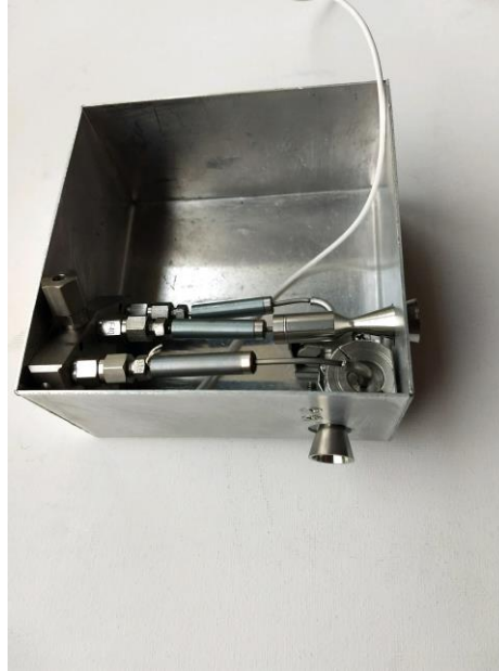
Cubesat tridyne/cold gas thruster triad system
