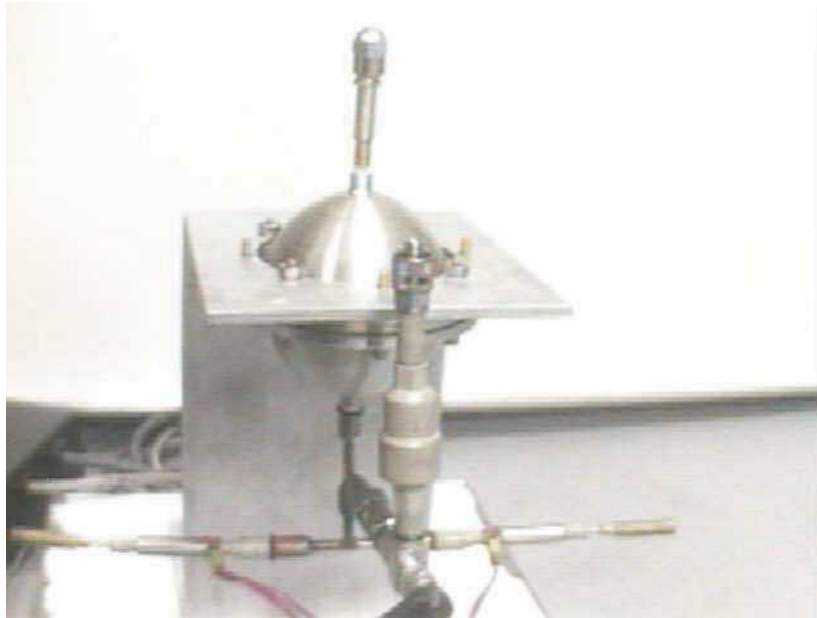
Thruster Module with 2-inch Tank, micro-solenoid valves and thrusters
